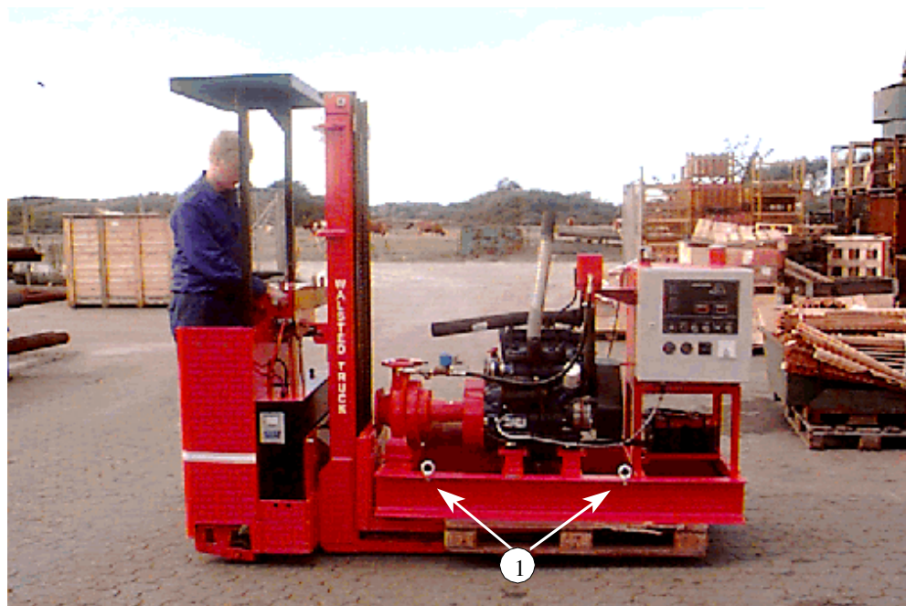
Figure 1: Transportation of sprinkler system, 1) Lifting eyes
